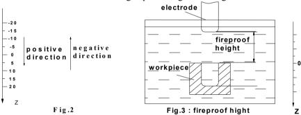
DRO for EDM provides fireproof function. During EDM, charcoal will be produced on the machined surface. With accumulating charcoal, the electrode will beyond liquid level, which could lead a fire. If fireproof height is set, EDM will stop, the DRO will send an alarm and fire is avoided.
