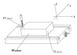
In horizontal plane, the X axis is parallel with the operator; Y axis is perpendicular to X axis. Z-axis is perpendicular to horizontal plane. Positive direction of axis is set as the figure. It also can be changed as customer.
