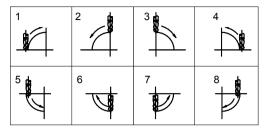
Tool compensation direction (when process XY plane)
