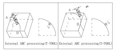
Milling cutter may be flat-bottomed or arc-bottomed. If flat-bottomed, set the tool diameter as 0;
